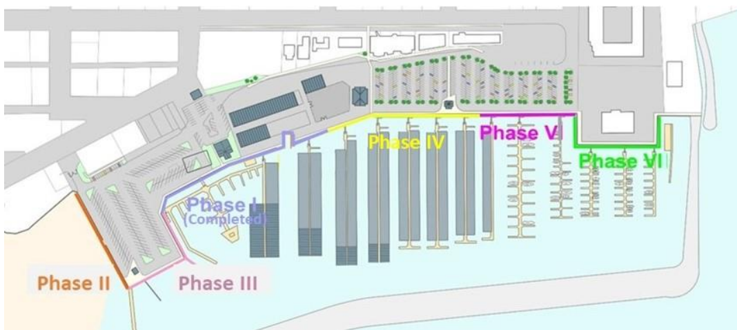
Figure 4-1. Bulkhead Replacement Phasing
