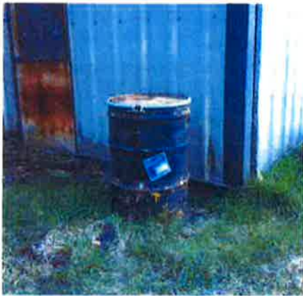
(BEFORE) Photo 02: STORAGE BARREL CONTAINING UNKNOWN MATERIAL UNCOVERED AND WITHOUT SECONDARY CONTAINMENT
