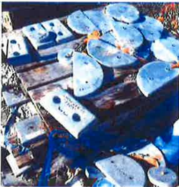
(BEFORE) Photo 02: NW CORNER MATERIAL STORAGE. MARITIME ZINCS (SACRIFICIAL ANODES) EXPOSED TO RAINFALL.
