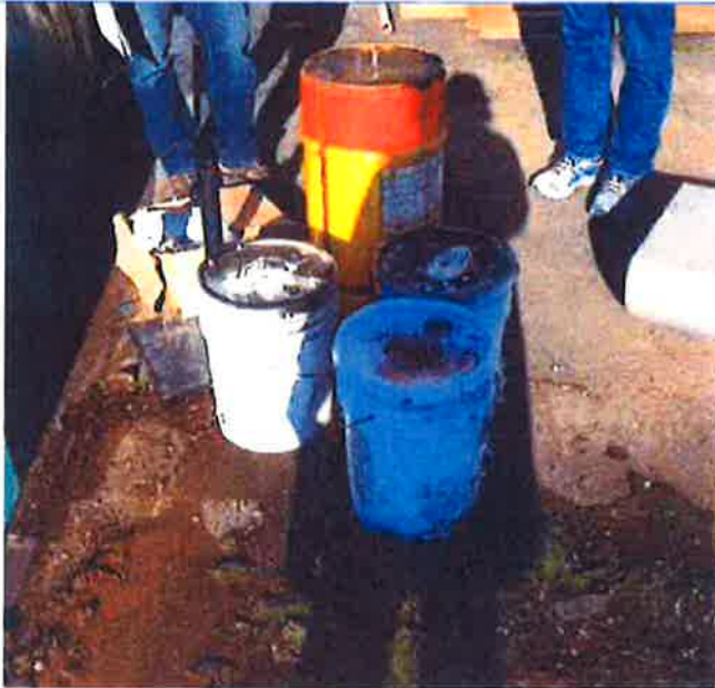
(BEFORE) Photo 14: CONTAINERS ON LOADING PLATFORM EXPOSED TO RAINFALL.
