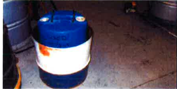
(AFTER) Photo 01-A: USED ANTIFREEZE BARREL HAS BEEN REPLACED AND MOVED INSIDE MECHANIC SHOP UNDER COVER WITH SECONDARY CONTAINMENT AND LOCATED CLOSER TO THE SPILL KIT
