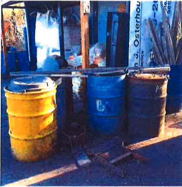
(BEFORE) Photo 07: SOUTH FENCELINE MATERIAL STORAGE. POLLUTION GENERATING MATERIAL EXPOSED TO RAINFALL. SAND BAGS UNDER COVER TO PREVENT DETERIORATION.
