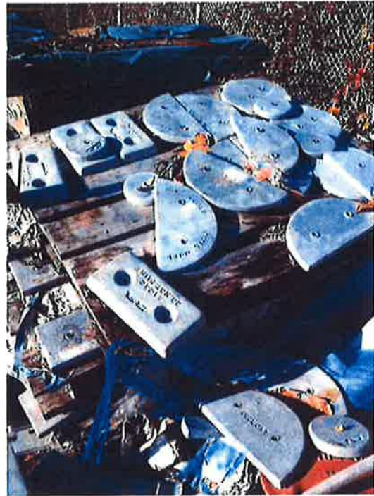
02 DESCRIPTION: NW CORNER MATERIAL STORAGE. MARITIME ZINCS (SACRIFICIAL ANODES) EXPOSED TO RAINFALL.
