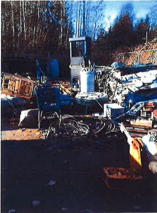
01 DESCRIPTION: NW CORNER MATERIAL STORAGE. POLLUTION GENERATING MATERIAL EXPOSED TO RAINFALL.
