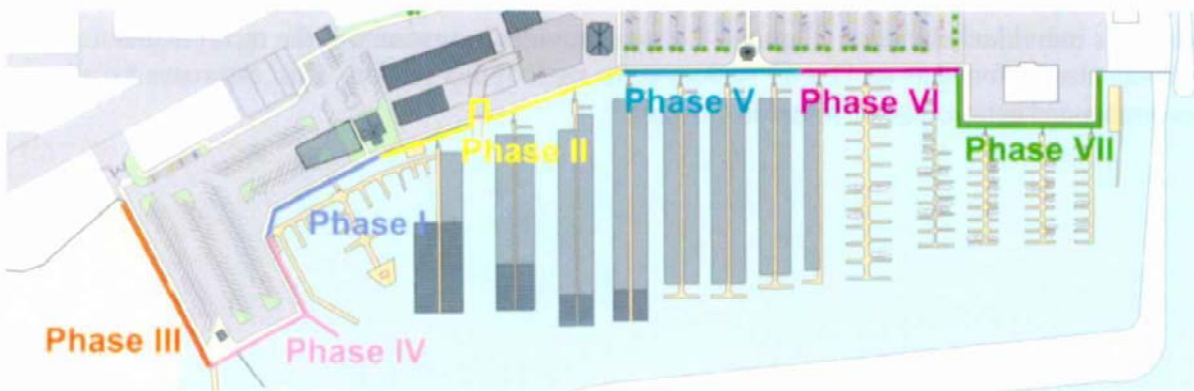
Figure 4-2. Bulkhead Replacement Phasing
