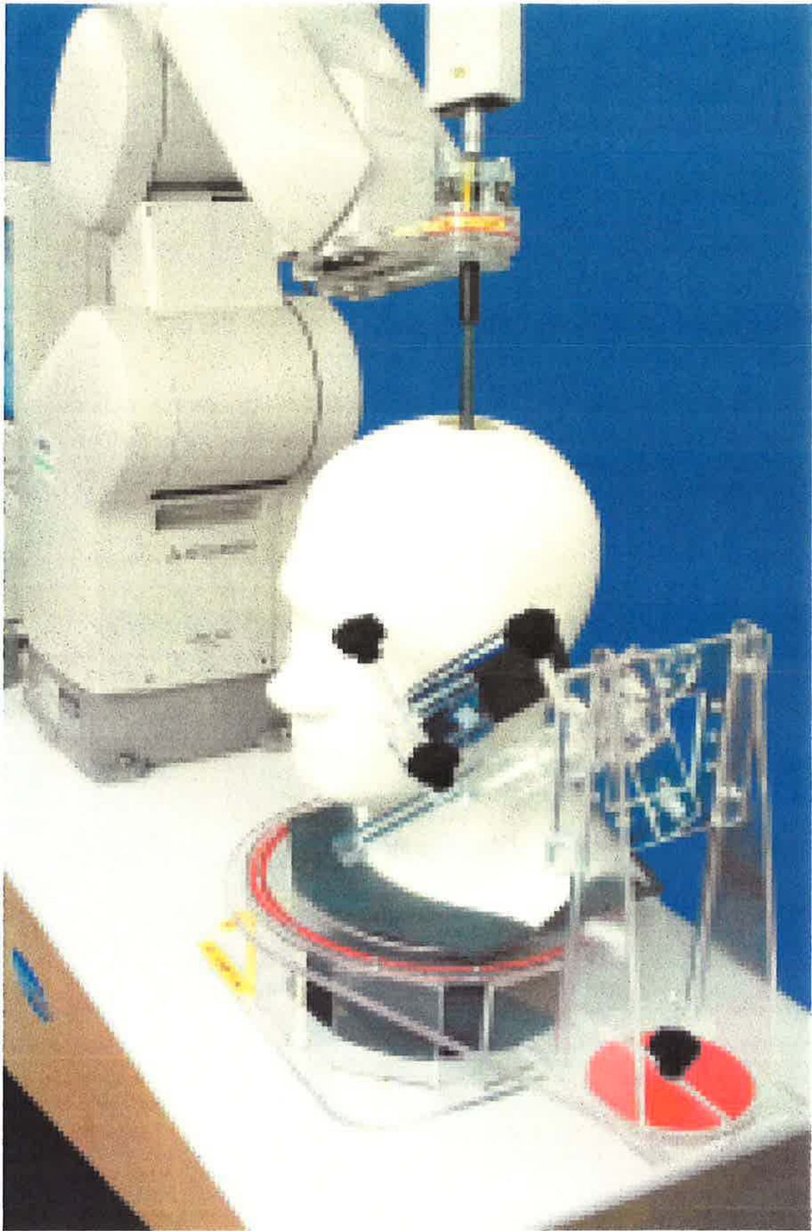
SAM (Specific Anthropomorphic Mannequin) Phantom head for SAR test (Specific Absorption Rate c. 1996)
