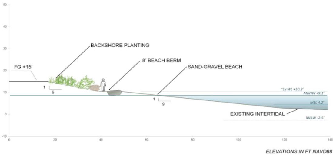
TYPICAL BEACH SECTION DES MOINES CREEK ESTUARY RESTORATION
