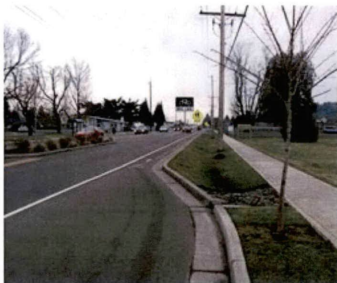
LID ELEMENTS: CURB INLETS, RAINGARDENS, CURB BULBS WITH PARKING, CENTER ISLAND LANDSCAPING
