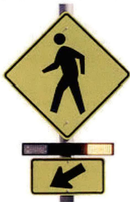
Rectangular Rapid Flashing Beacon (RRFB)
